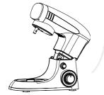
2. Push the arm release button (3). at the same time lift the swivel arm(2) so that it locks into place with a click, The swivel arm tilts up.
