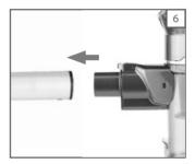
3. Remove the accessory adapter (10) from the suction nozzle by pressing the suction nozzle release button (4) (Fig 7).
